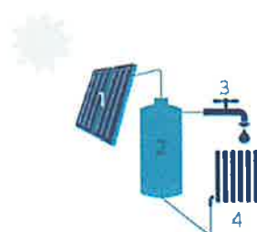
Diagram illustrating the connection of a solar collector (1) to a storage tank (2) and a radiator (4).
